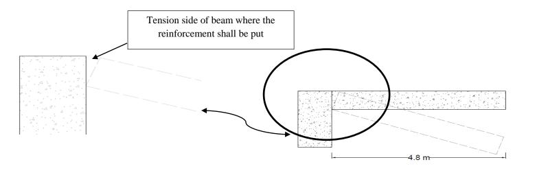
Example: check the adequacy of a simply supported beam shown in figure below when subjected to a factored load of Wu=70 kN/m (including self-weight), use fc = 28 Mpa and fy=420 Mpa
