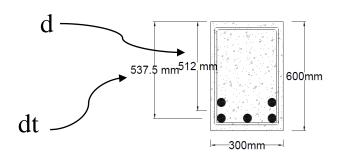
Example: for the precast beam shown in Figure below, the designer intended to use  $4\phi20$  ,check the adequacy of the beam according to ACI requirement, the beam is subjected to uniform dead load (15) kN/m (with self-weight) and uniform live load (20) kN/m
